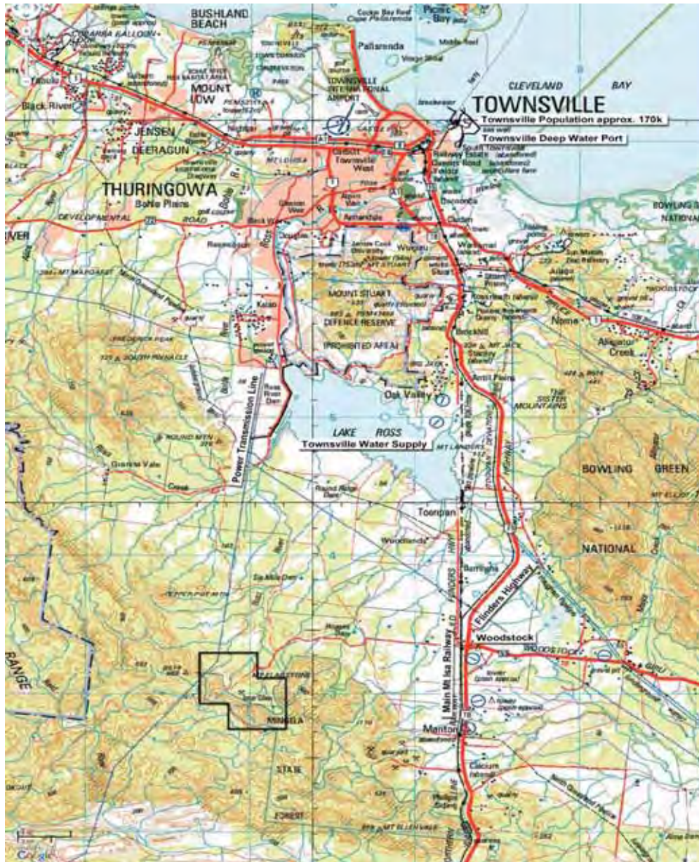
Figure 5 - Section of Topographic Sheet (100,000 topographic sheet (#8258)), showing Iron Glen Tenement and Infrastructure (roads, railroad, power line, creeks, and the Mingela State Forest)
